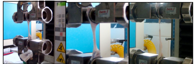
Figure 13. (A) Tensile strength test was conducted by using the Zwick universal tensile strength testing machine , (B) The skin was intact ( early phase), (C) The skin was broken ( end phase)
